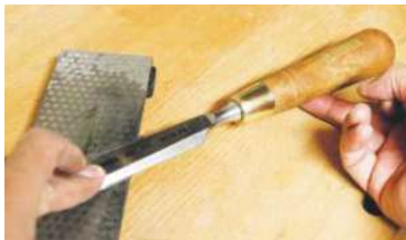
▲ Importantly, it also lifts the stone high enough so that chisel handles are clear
